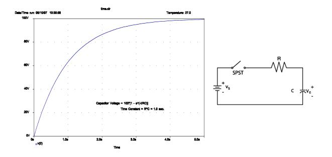
Graph of capacitor voltage (vc) versus time
