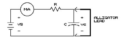
2. Record the initial current reading of the milliammeter; it should be closed to "full-scale" for a digital meter on the 2 mA range (I = [30 V/16 k $\Omega$ ]). Express the current in units of  $\mu$ A.
